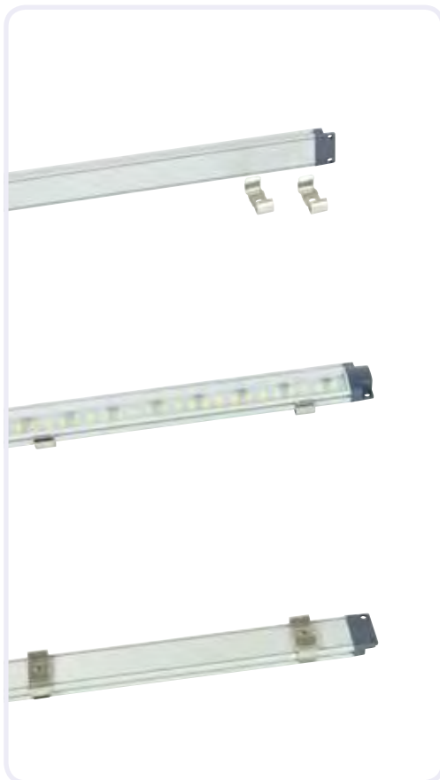
The LED can be mounted in 3 ways. By screwing, double-sided taping or by using the mounting clips. All of these mounting materials are also supplied as standard.
